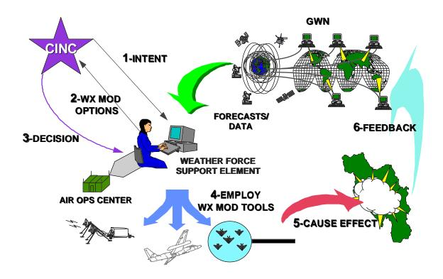
Figure 3-2. The Military System for Weather-Modification Operations.
