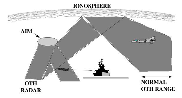
Figure 4-3. Artificial Ionospheric Mirror Over-the-Horizon Surveillance Concept.
