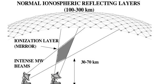
Figure 4-1. Crossed-Beam Approach for Generating an Artificial Ionospheric Mirror
