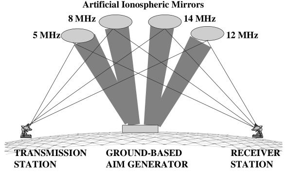
Figure 4-2. Artificial Ionospheric Mirrors Point-to-Point Communications
