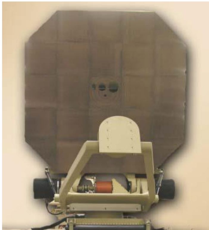
Figure 80. Active Denial System (ADS) Antenna (from Miller, NATO NAVAL ARMAMENTS GROUP 2009)
