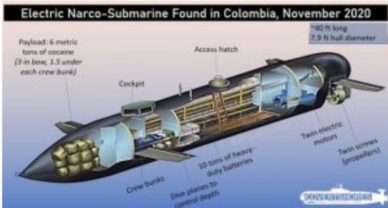
This “fully submersible electric-powered submarine makes it very hard to trace. The vehicle was capable of carrying 6 tons of cocaine. The street value of such a huge amount stands at an estimated \$120 million USD” (Kundu, 2020). Although not unmanned yet, it is clear to see that the narco-traffickers are working on undersea logistics to move their products. It will only be a matter of time before they add unmanned underwater vehicles to their fleet.
