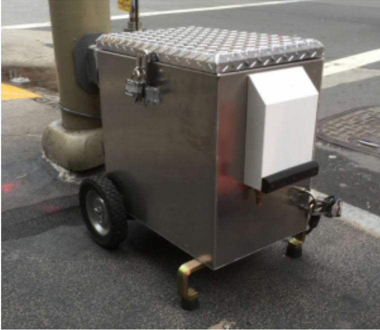
Biowatch Gen 2 detection capabilities consist of outdoor aerosol collectors whose filters are manually retrieved for subsequent analysis in a State or county public health laboratory that is a member of the CDC Laboratory Response Network. The results are generally received 8-10 hours after sample delivery to the laboratory. Biowatch Gen 2 is labor-intensive, and products may not be available until 12-36 hours after a biological agent's release has occurred. (See Figures 10-3 & 10.4)
