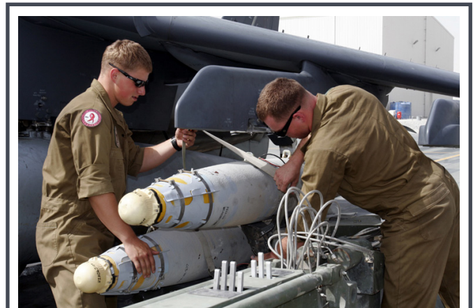
Ordnance technicians with the Marine Expeditionary Brigade-Afghanistan mount a Joint Direct Attack Munition to an AV-8B Harrier at Kandahar Airfield.
