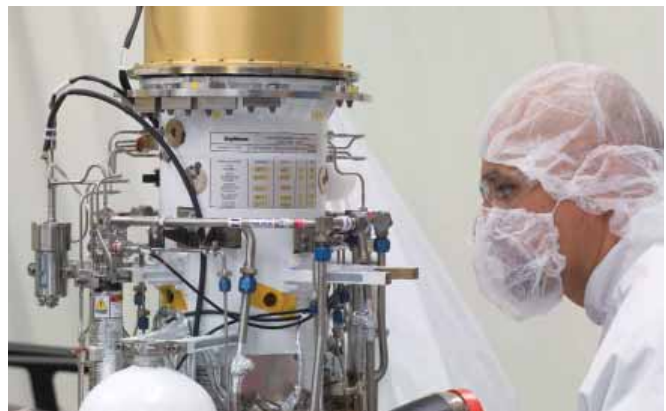
A RAYTHEON TECHNICIAN INSPECTS A HIGH-PRESSURE GAS LINE DURING ASSEMBLY OF AN EXOATMOSPHERIC KILL.
